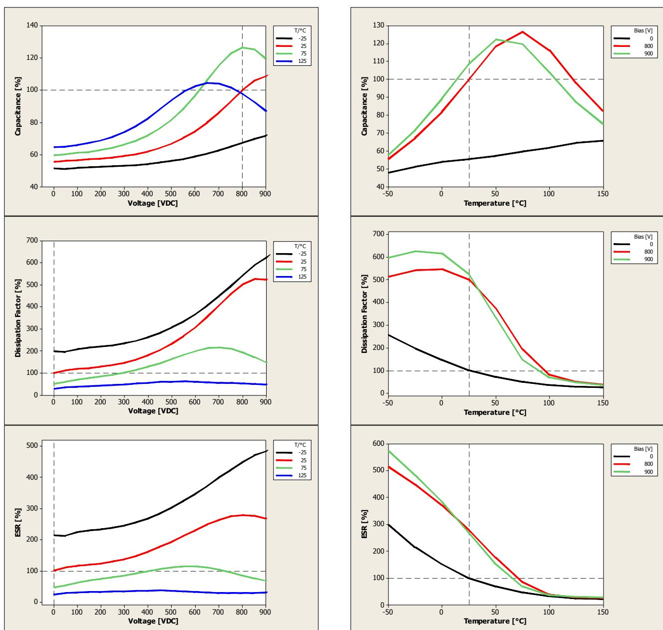
**Typical capacitance values as a function of voltage  $V_R = 900$  V**
