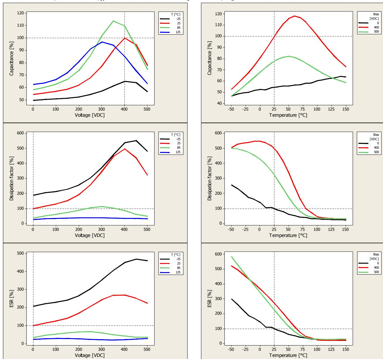
**Typical capacitance values as a function of voltage  $V_R = 500$  V**
