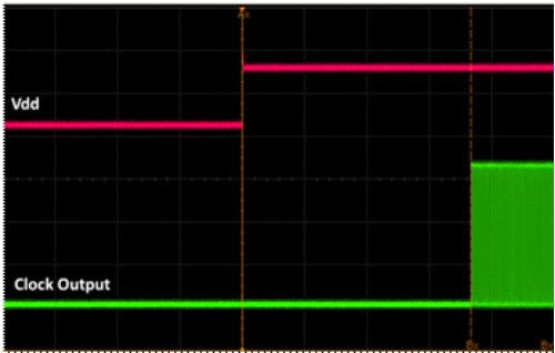
Figure 16. Startup Waveform vs. Vdd
