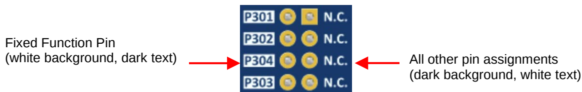
Figure 23. Fixed Function Pin Label Example
